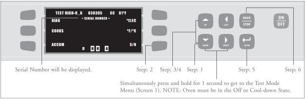
FIGURE 38: Viewing/Entering the Serial Number
